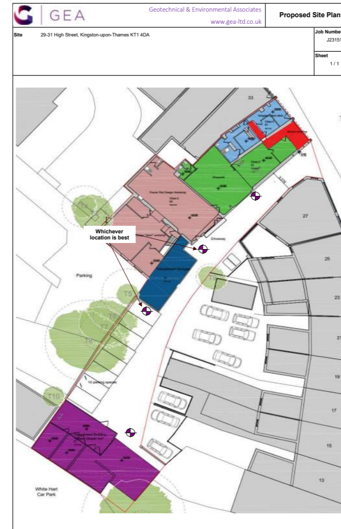
Figure 4.1- Borehole locations- Refer to Appendix A for original
