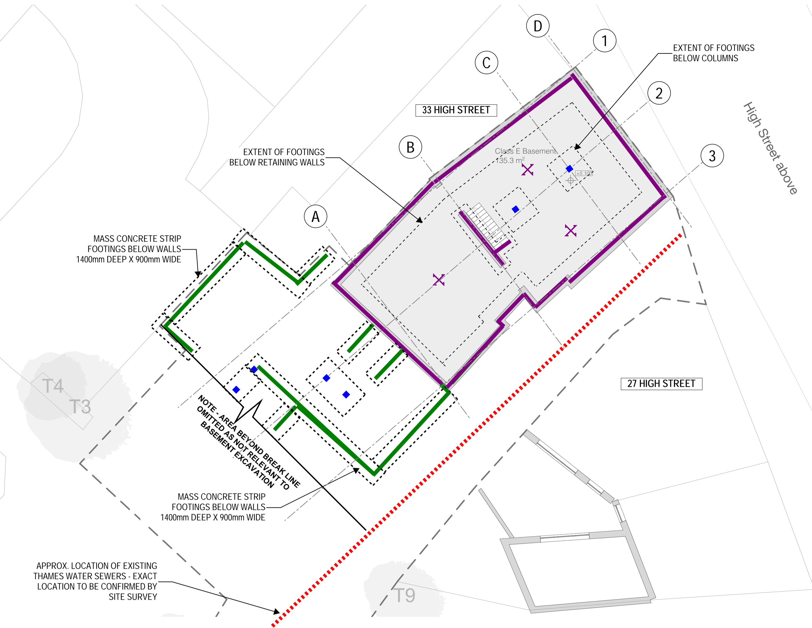
PROPOSED BASEMENT PLAN EXTRACT FROM ARCHITECTURAL DRAWING TP(10)20 MINOR OPENINGS FOR WINDOWS, DOORS ETC. OMITTED FOR CLARITY, MAKE SUITABLE ALLOWANCE FOR LINTELS N.T.S.
