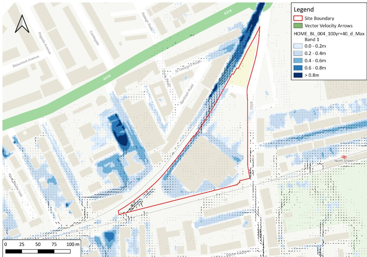
Figure 6. Baseline Modelling - 1 in 100-year plus 40% Climate Change Maximum Depths and Velocity
