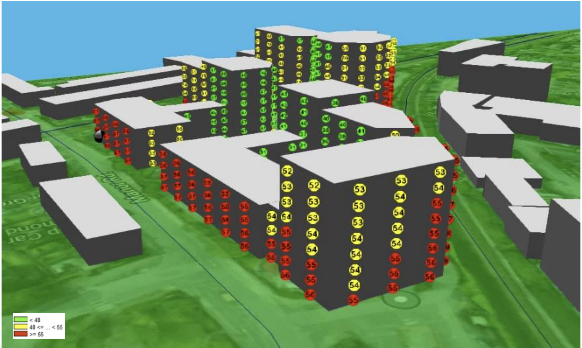
389 Manor Road, Richmond Facades Overlooking Manor Road - Night-time Levels and Criteria Project 11695
