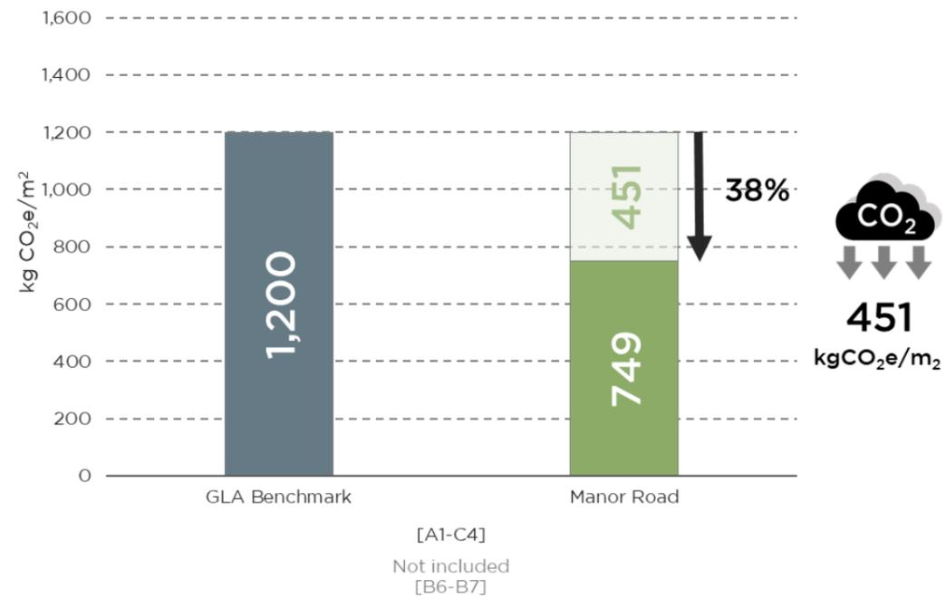
Figure 1.2 - Total embodied carbon over the life-cycle against GLA WLC benchmark
