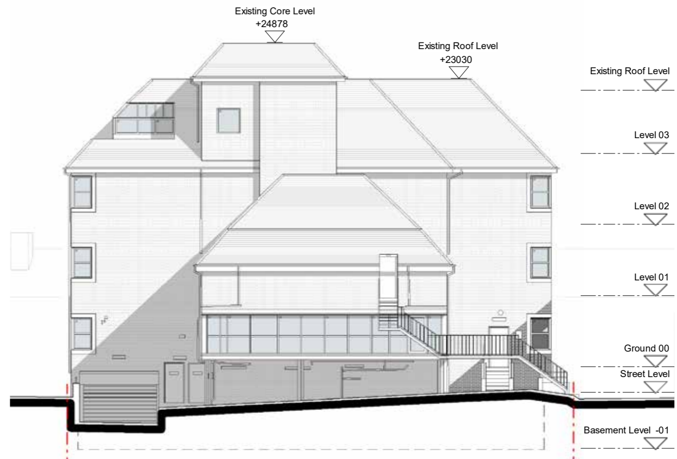
Existing South Elevation
