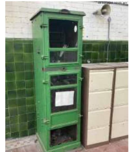
Harland control cabinet for electric centrifugal pump
