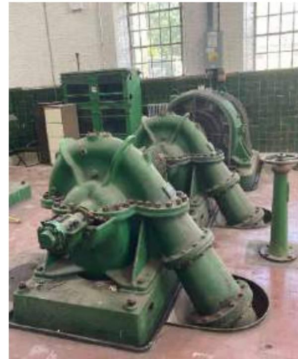
Harland twin impeller electric centrifugal pump set
