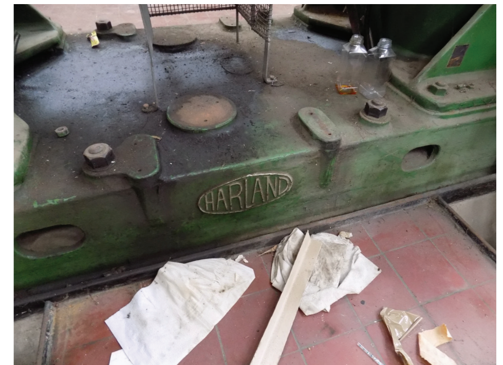
Figure 21: Bedplate detail: 1932 Harland twin impeller electric centrifugal pump set, Ruston & Ward Engine House (low to medium significance)
