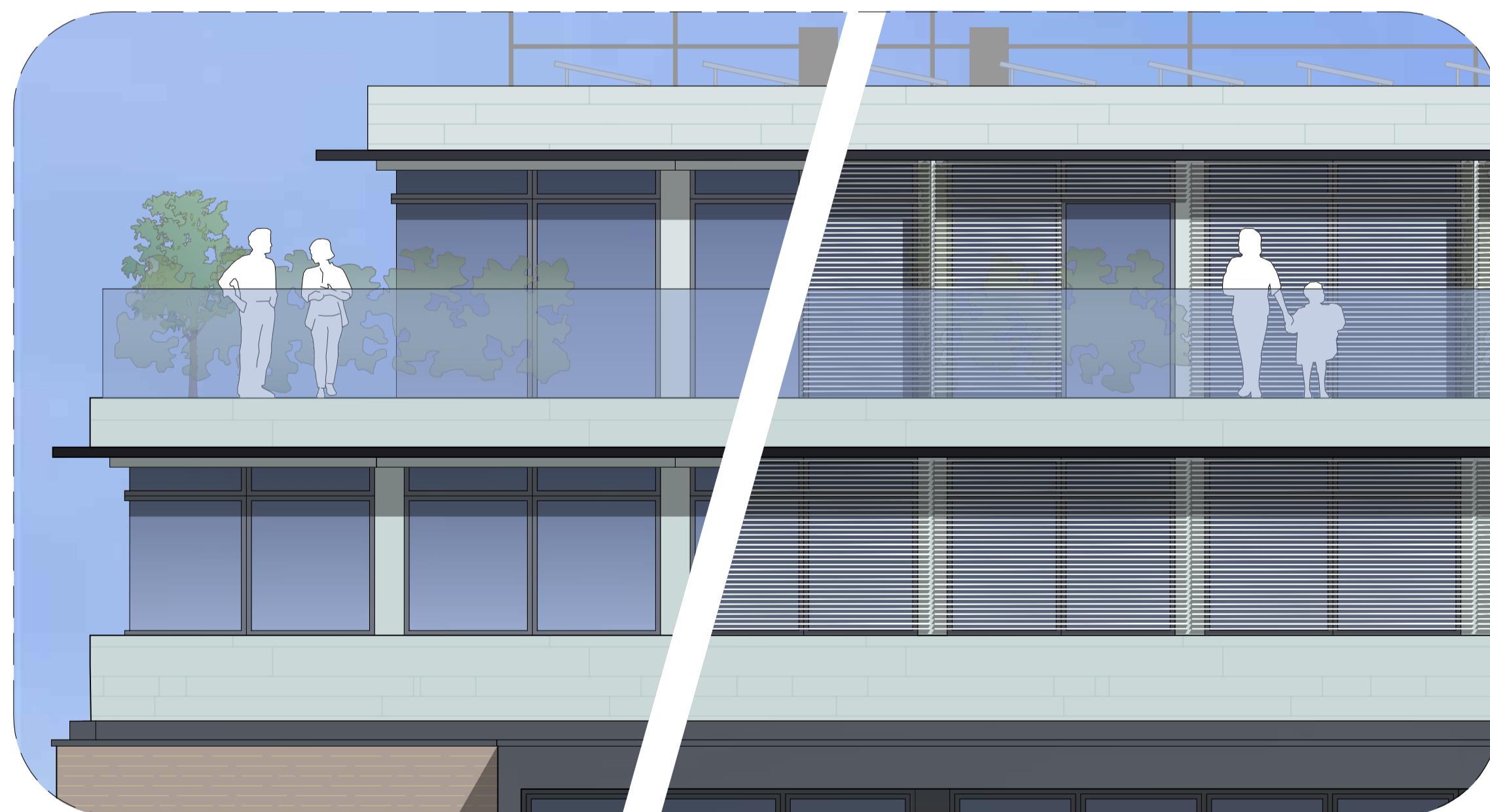
3 EXTRACT SHOWING BLINDS UP Vs DOWN 1 : 50
