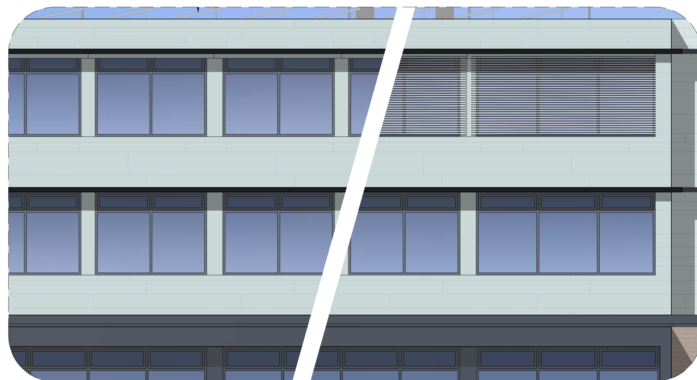
3 EXTRACT SHOWING BLINDS UP Vs DOWN 1 : 50
