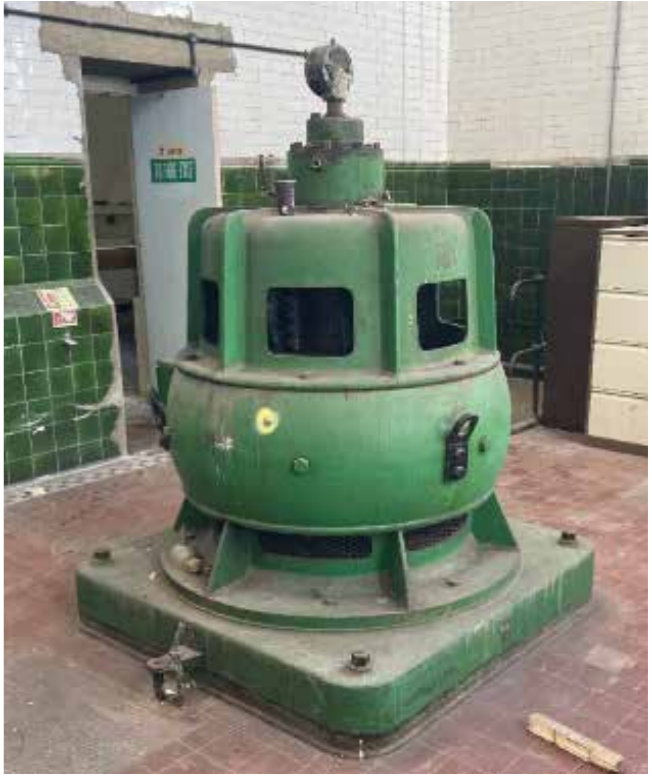
Harland DC Motor Date: 1932 Size: 1.6m x 1.6m Report comment: Low to medium significance
