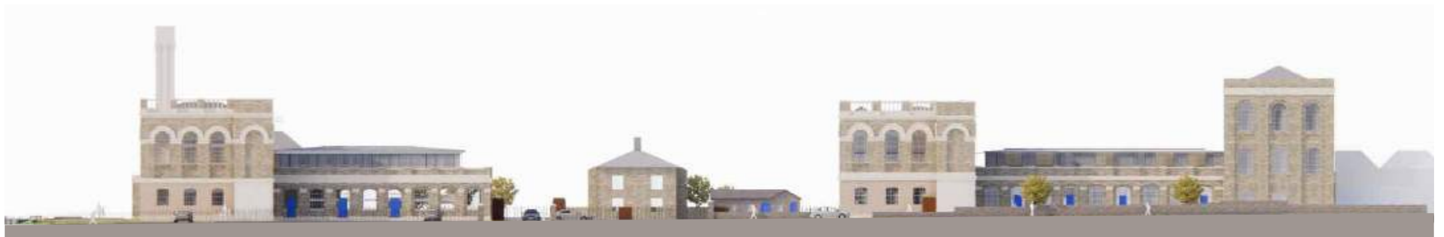
Current proposal - Roof extensions refined and cottage extension reduced to single storey
