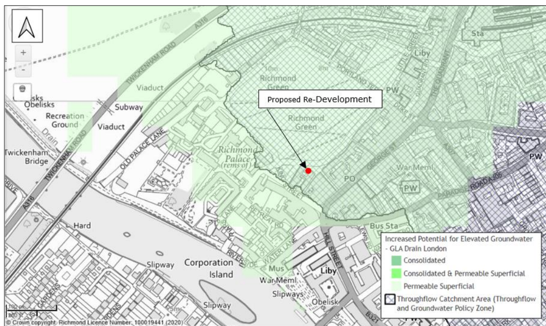
Figure 4-4: Increased Potential for Elevated Groundwater and Throughflow Catchment Area (Source: London Borough of Richmond upon Thames Interactive Maps, SFRA 2021)
