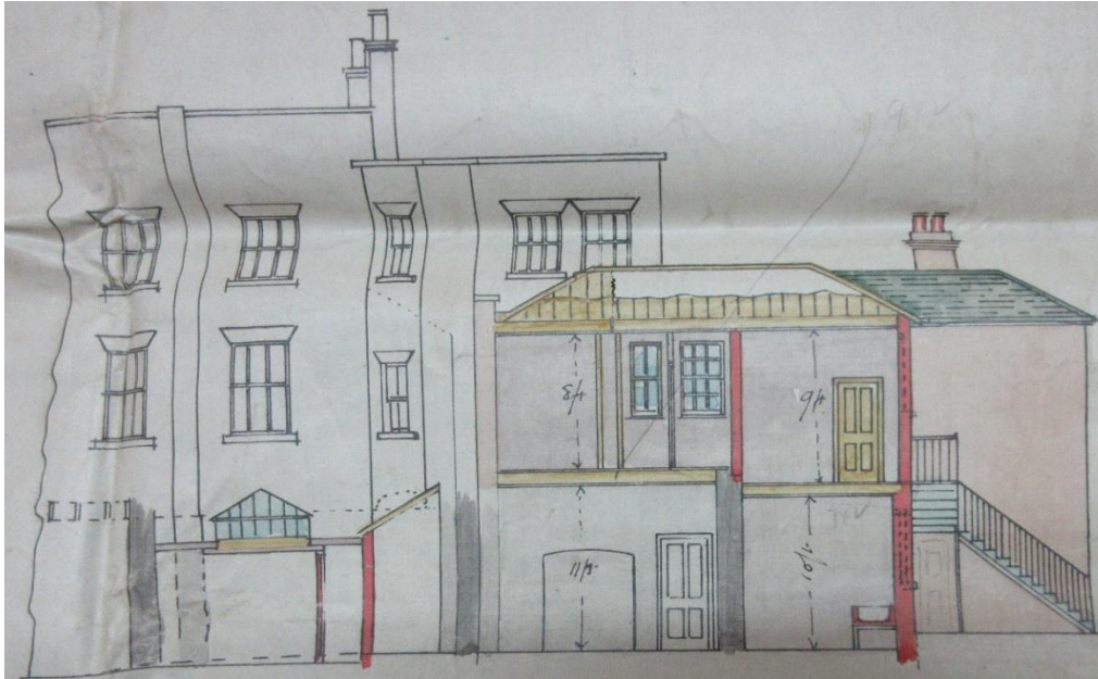
Figure 53: Section AB – proposed two-storey extension to the rear of George House, including re-modelled kitchens and new bedrooms, 1920.
