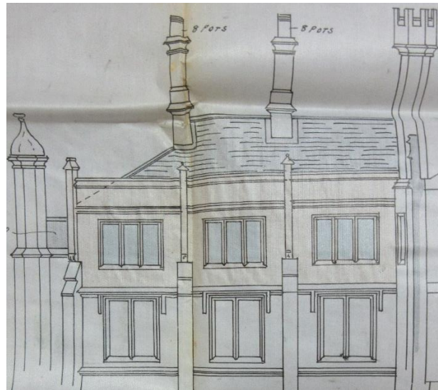
Figure 45 (left): Proposed end elevation of both north and south wings at second and third floor level, 1903.
