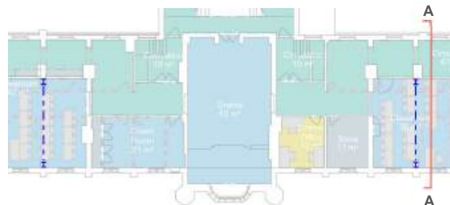
Extract from SK73 showing locations of proposed steel frames at 2 nd floor
