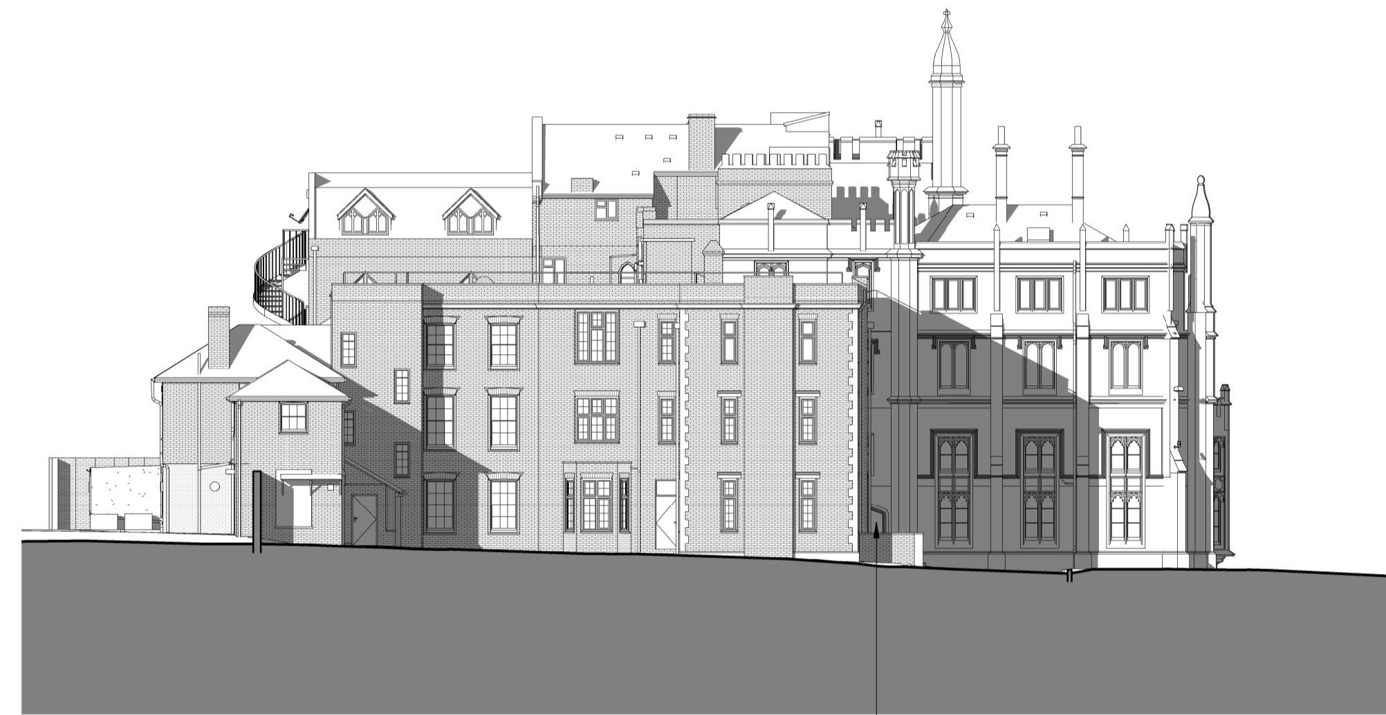
3 Main Building South East Elevation - Proposed 1:200
