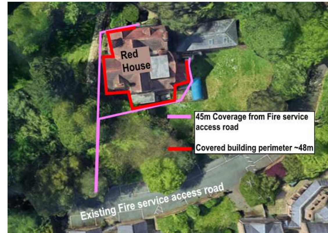
Figure 8-5: BS 9999: Red House Fire service access (reference – Google maps)
