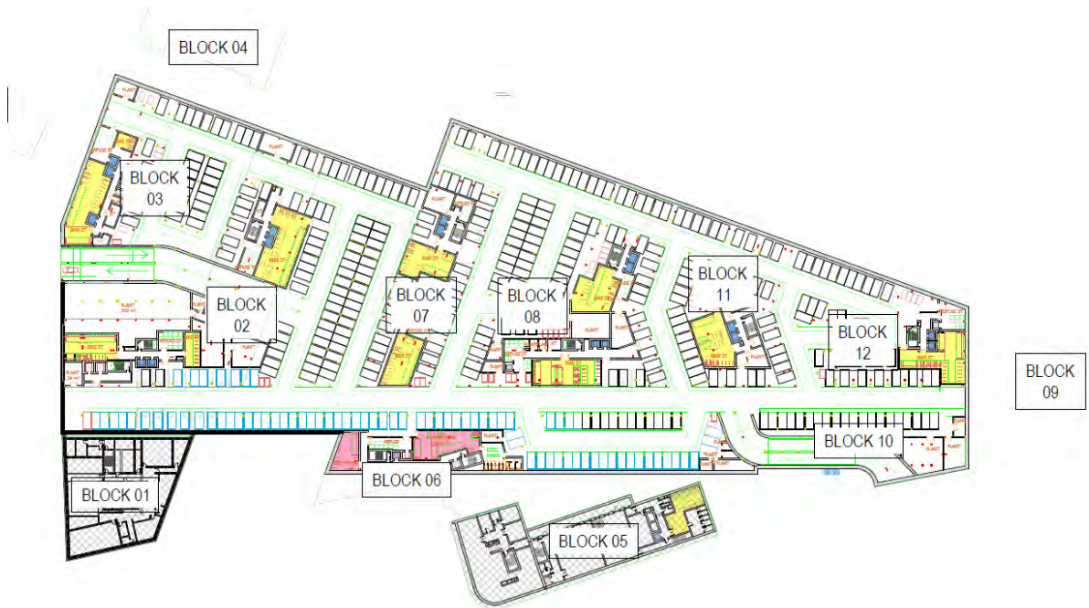
Figure 6-8: Basement Cycle Parking Stores (eastern basement, Development Area 1)
