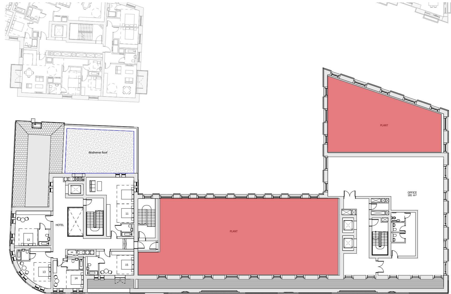
Location of Air Source Heat Pump plantrooms on upper floors of Building 5
