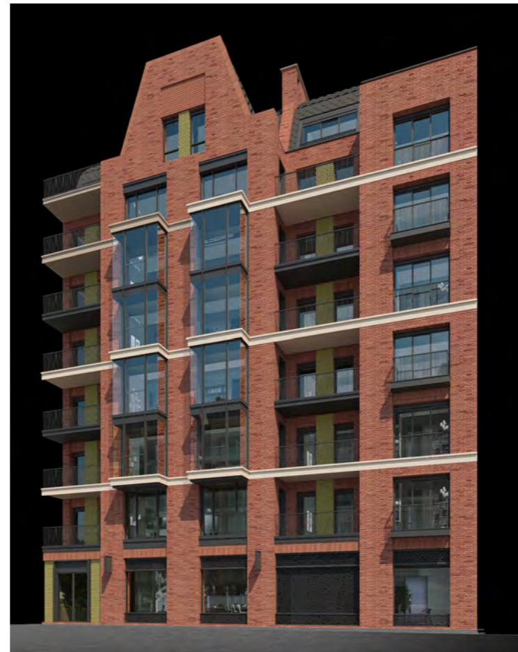
Bay Study showing variation in brickwork colour - Courtyard 2
