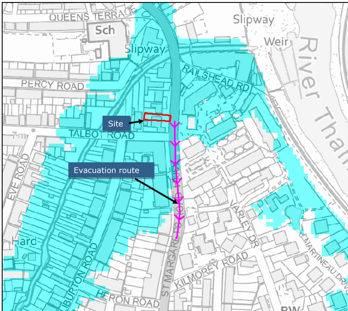
Figure 7: Preferred evacuation route in relation to Breach inundation map for 2100 (taken from Thames_Upriver_Breach_Model_P6)
