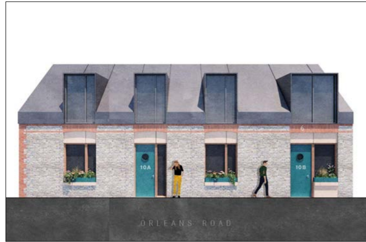
1. Above, first thoughts & initial elevations showing large roof dormers and dual entrances along Orleans Road. Metal roof cladding and square format opening windows. Below, testing plan options for a larger single home rather than two dwellings.
