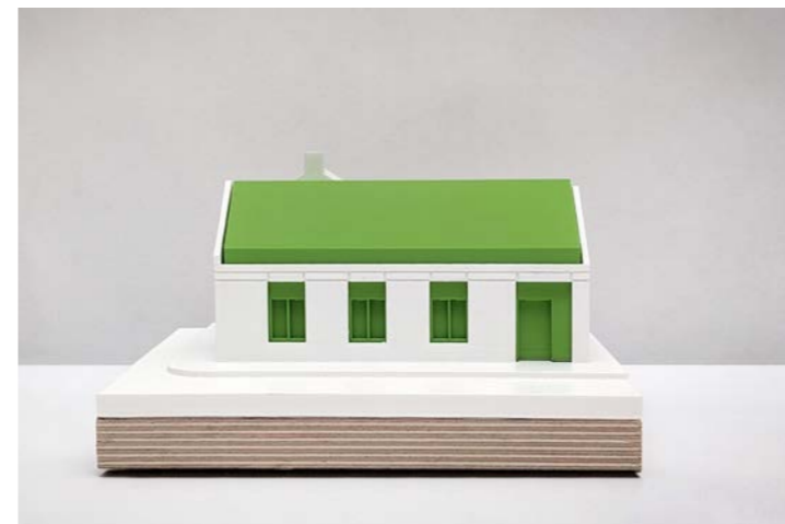
Group dormers and ground floor windows together to give a lower eave height to upper floor
