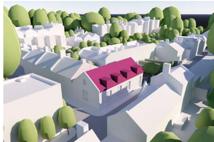
2. Following pre-app meeting the team looked at options to reduce the size of the roof dormers and tested the visual impact from street level to ensure no adverse impacts on townscape & the character of the area.
