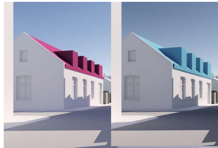
1. Above, first thoughts & initial elevations showing large roof dormers and dual entrances along Orleans Road. Metal roof cladding and square format opening windows. Below, testing plan options for a larger single home rather than two dwellings.
