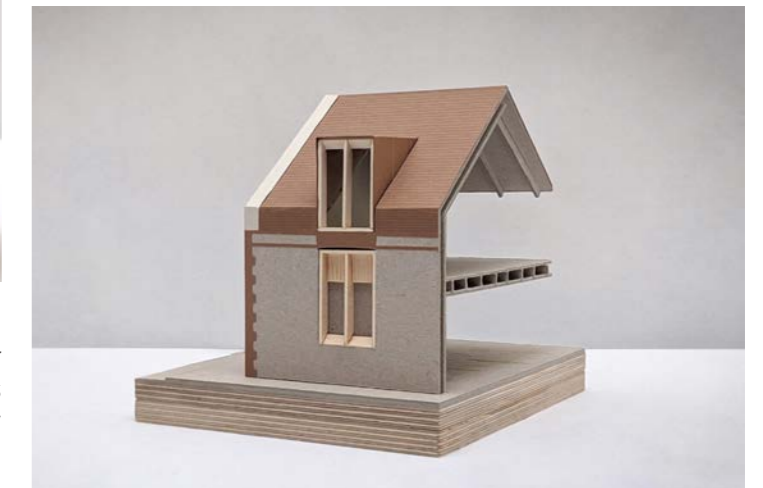
Group dormers and ground floor windows together to give a lower eave height to upper floor
