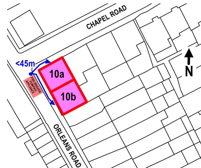
Figure 1. Fire Service Access within Site
