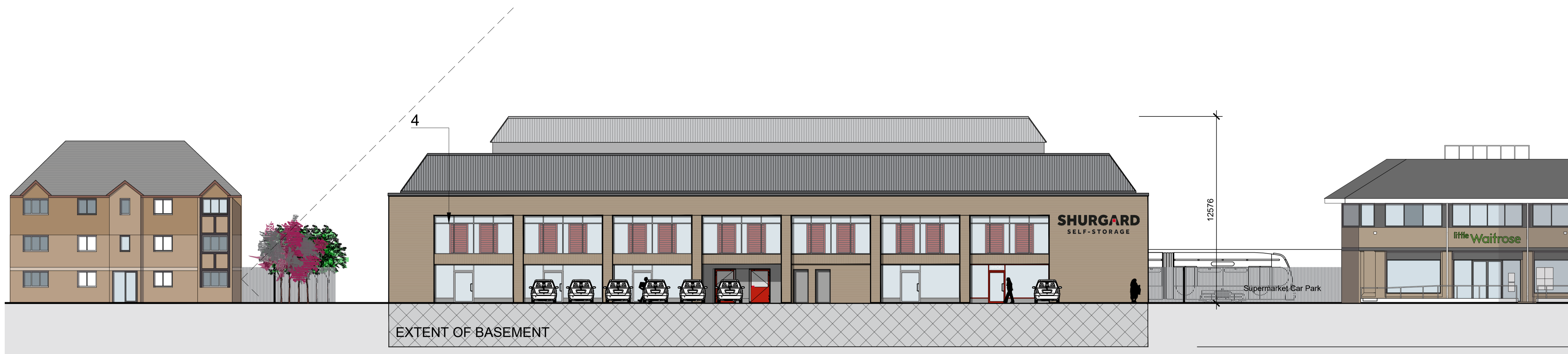
SOUTH ELEVATION TO THE OLDFIELD ROAD
