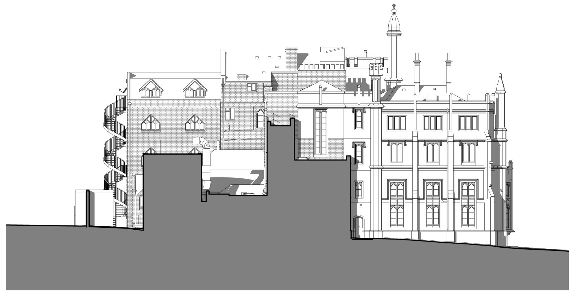
1 Main Building Section AA - Existing 1:200
