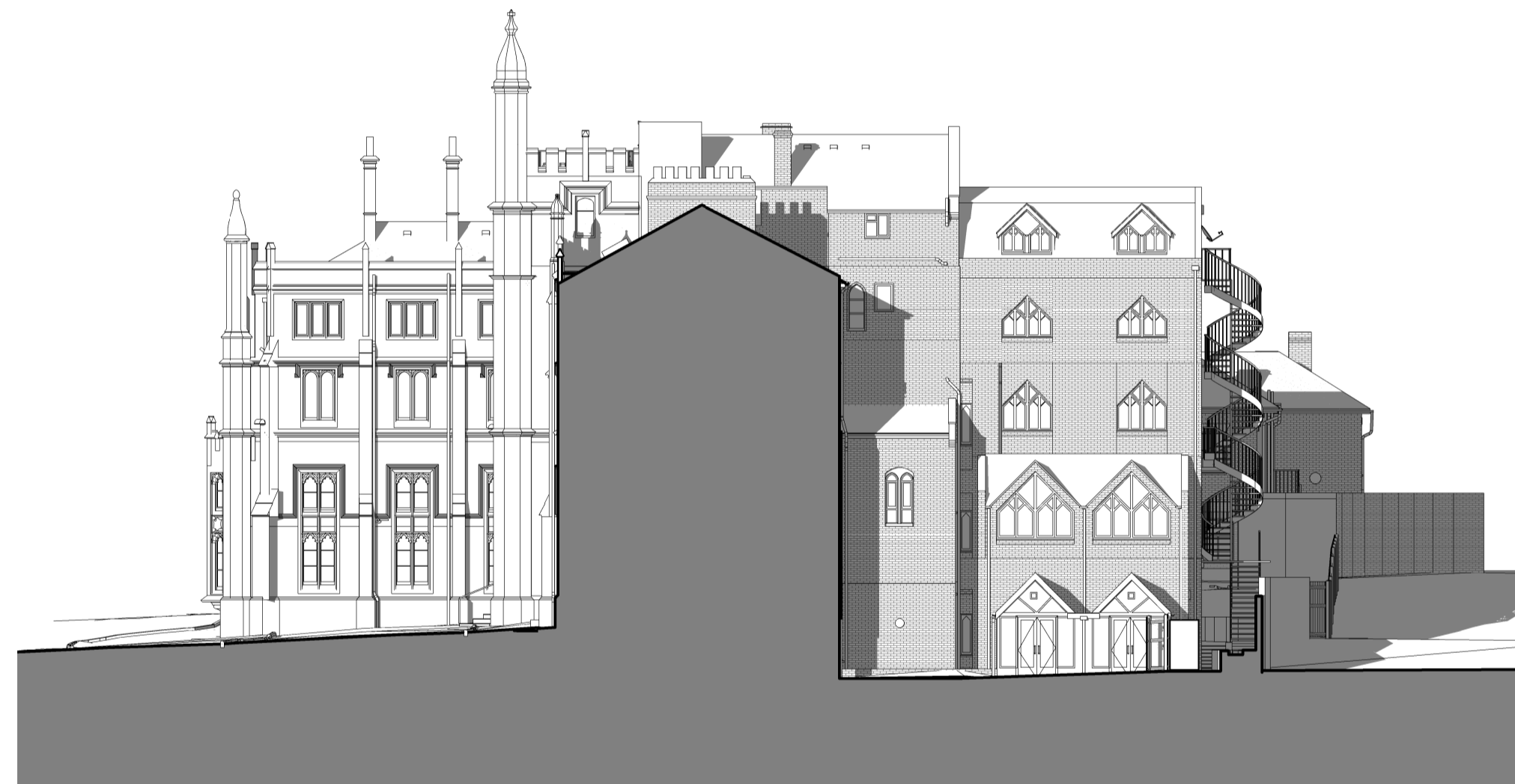
4 Main Building Section DD - Existing 1:200
