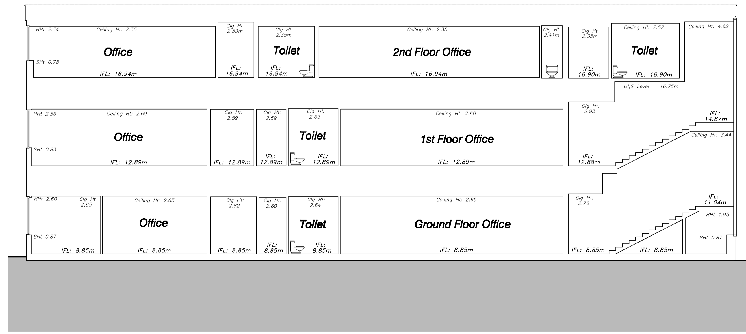
9. Long Section through building
