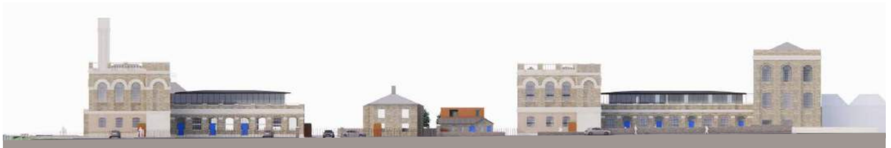
Iteration 1 - Roof extensions reduced to warehouses and cottages retained with two storey extension
