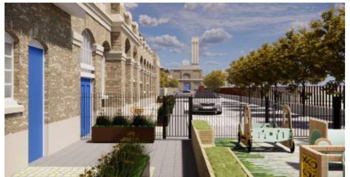
Shared Roadway Permeable block paving colour or size to be used to denote vehicle movement lines while providing pedestrian priority across the site.
