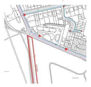
Additional fire hydrants are not proposed as the compartment does not exceed 280m² as per AD B Volume 2 Section 16.8 (noting that the ground and first floor are separate compartments).
