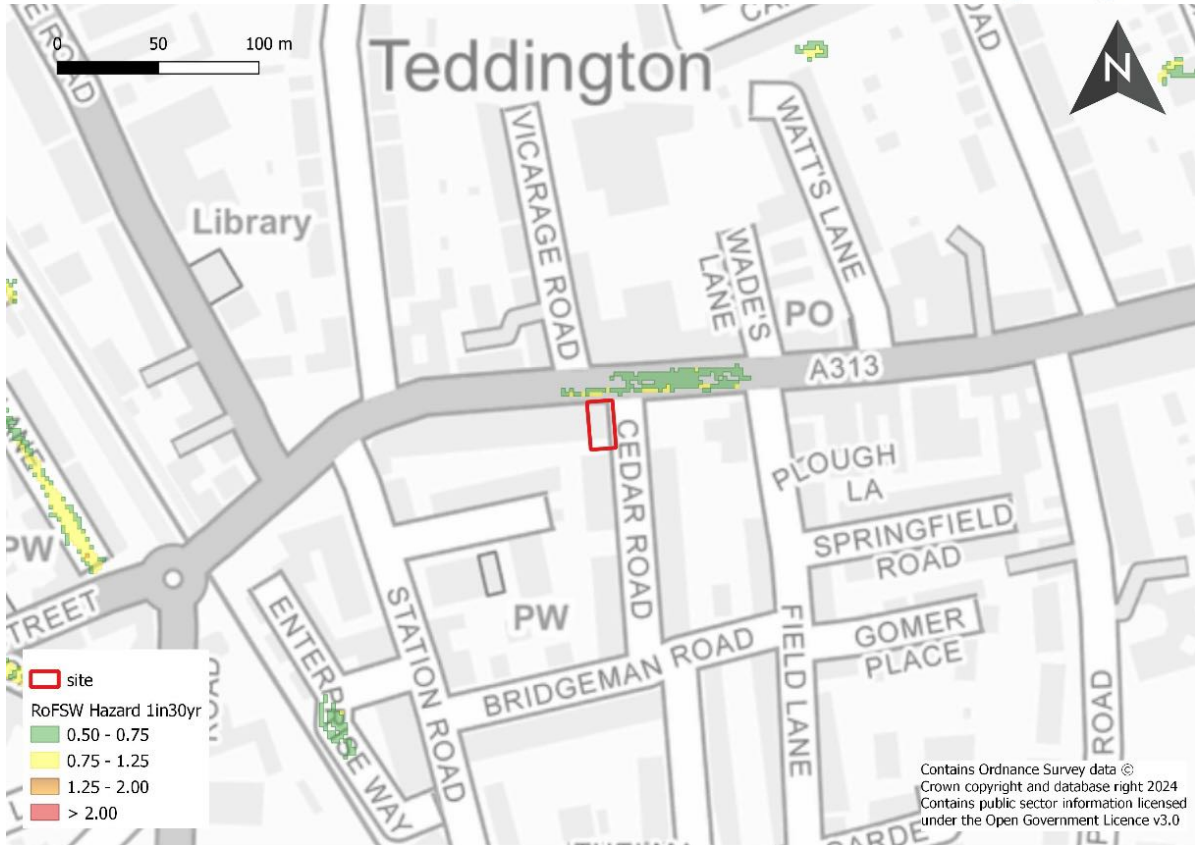
Figure 6: RoFSW Hazard Rating – High Risk (1 in 30 year)
