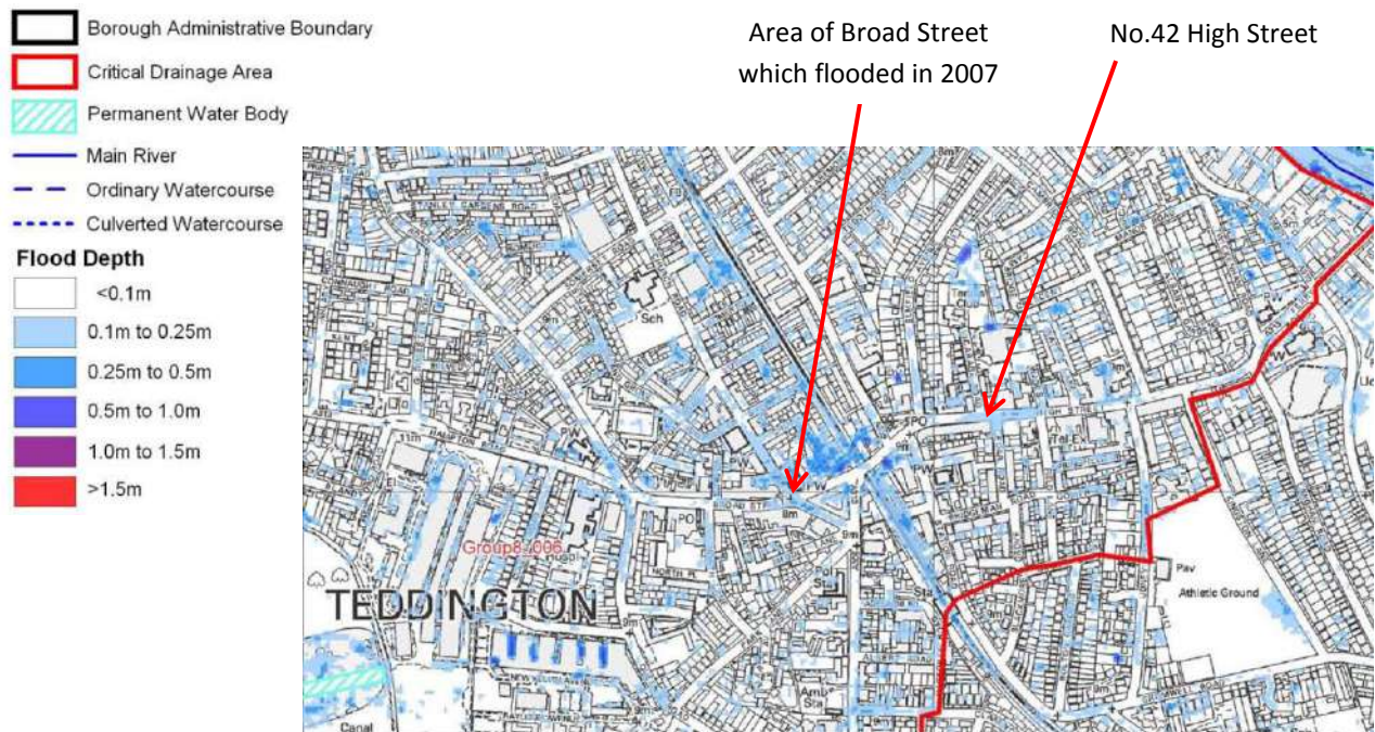
Figure 4: Enlarged extract from SWMP, Figure 3.8.6a: 'Group8_006 (Teddington). Surface Water Depth (m) 1 in 100 chance of rainfall event occurring in any given year (1% AEP)'. Ordnance Survey © Crown copyright 2011. All rights reserved. Licence No. 100051531.
