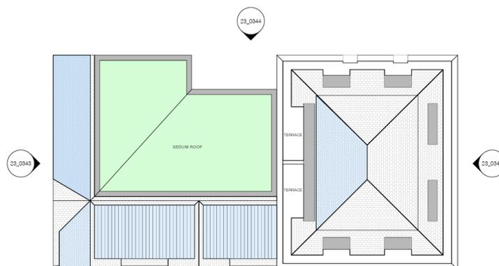
Figure 9: Proposed Roof Plan and PV Layout (Chandler Browne Architects)
