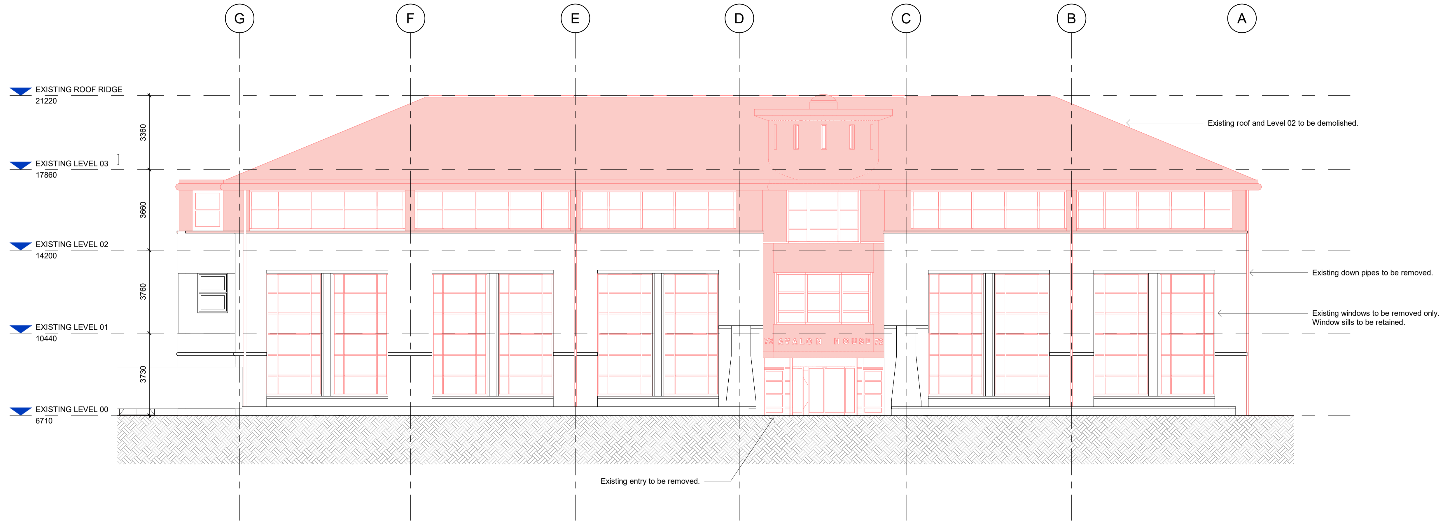
3 Demolition Elevation - North 1 : 100
