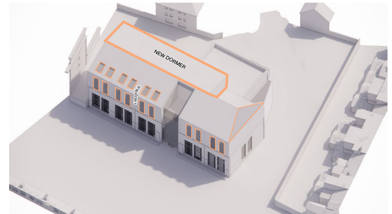
4. NEW WINDOWS, DORMER AND HIPPED ROOF
