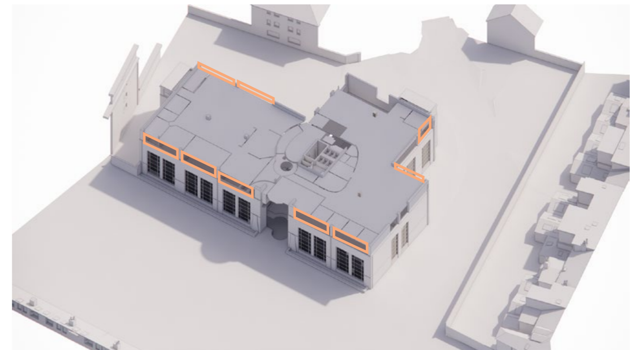
3. WINDOWS ON EXISTING SECOND FLOOR REMOVED
