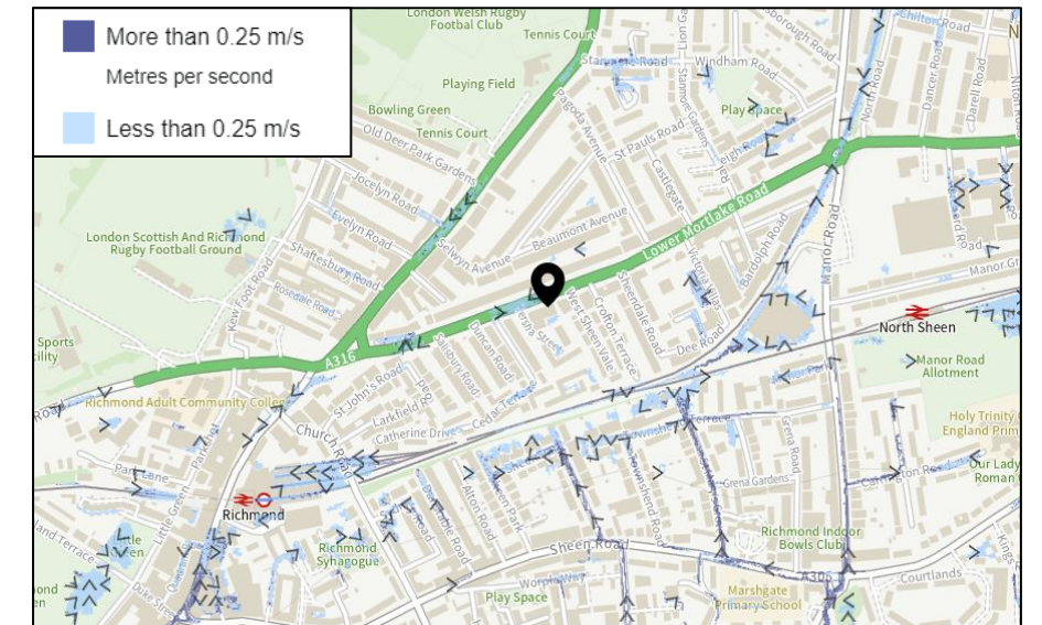
Figure 9: GOV.UK Flood Maps for Planning – Flood Risk from Surface Water: Water Velocity in a Medium Risk Scenario (1% chance each year)
