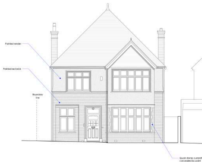
Existing Front Elevation
