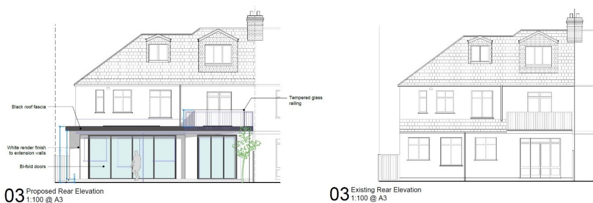
Figure 7 - Existing and proposed rear elevations
