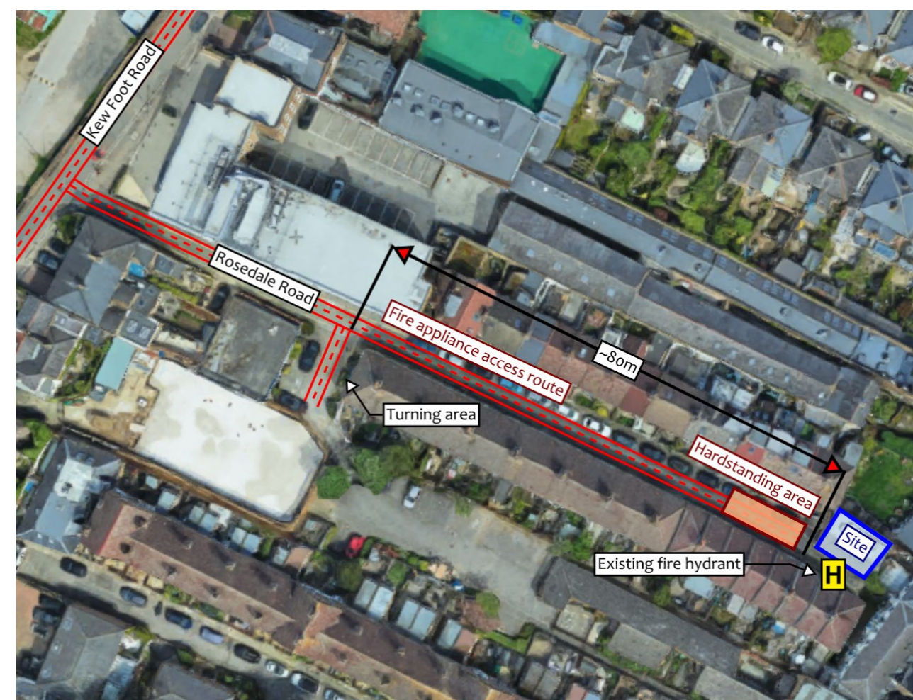
Figure 10 – Firefighting vehicle access and water supplies
