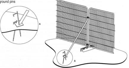
Figure 3b Stabiliser strut mounted on block tray
