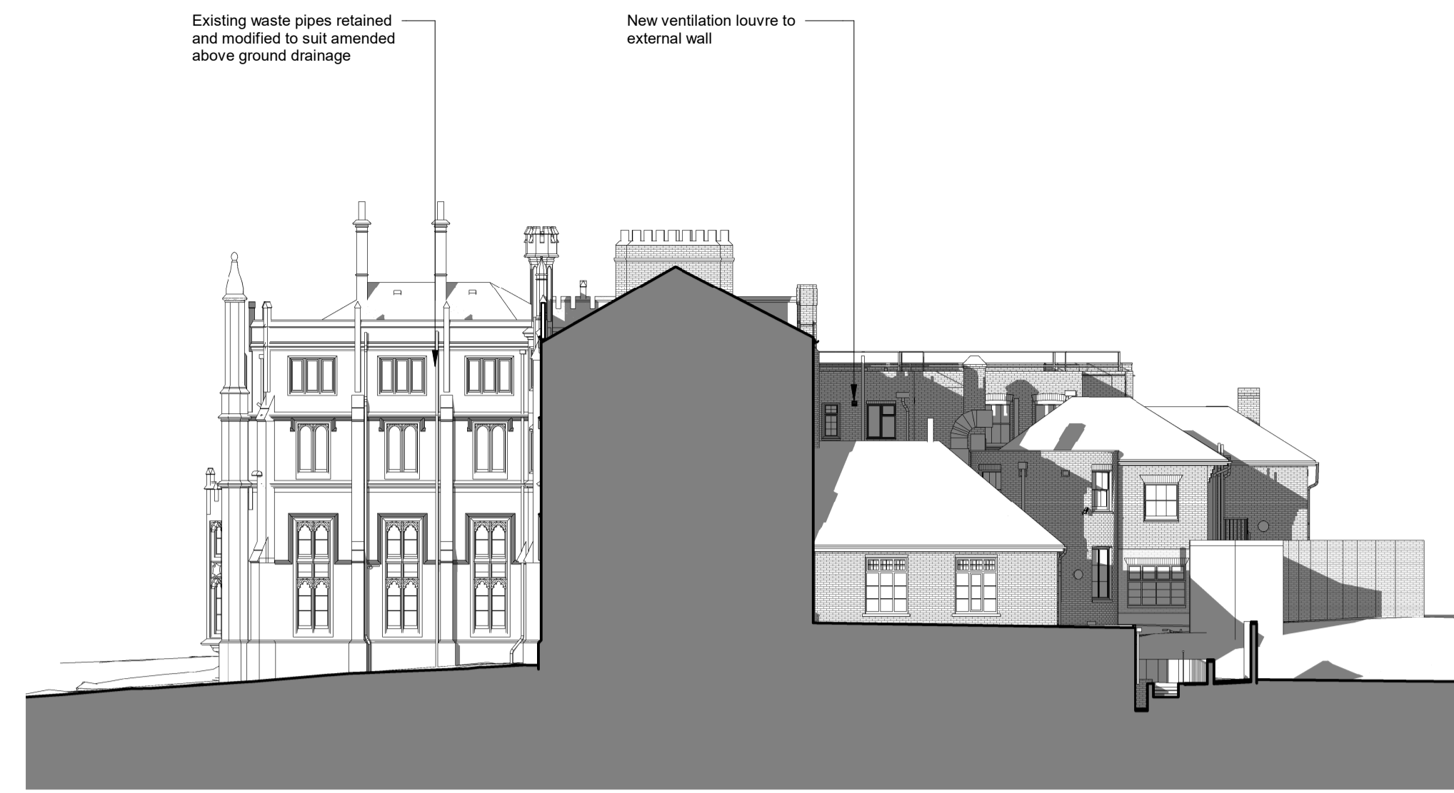
2 Main Building Section BB - Proposed 1:200
