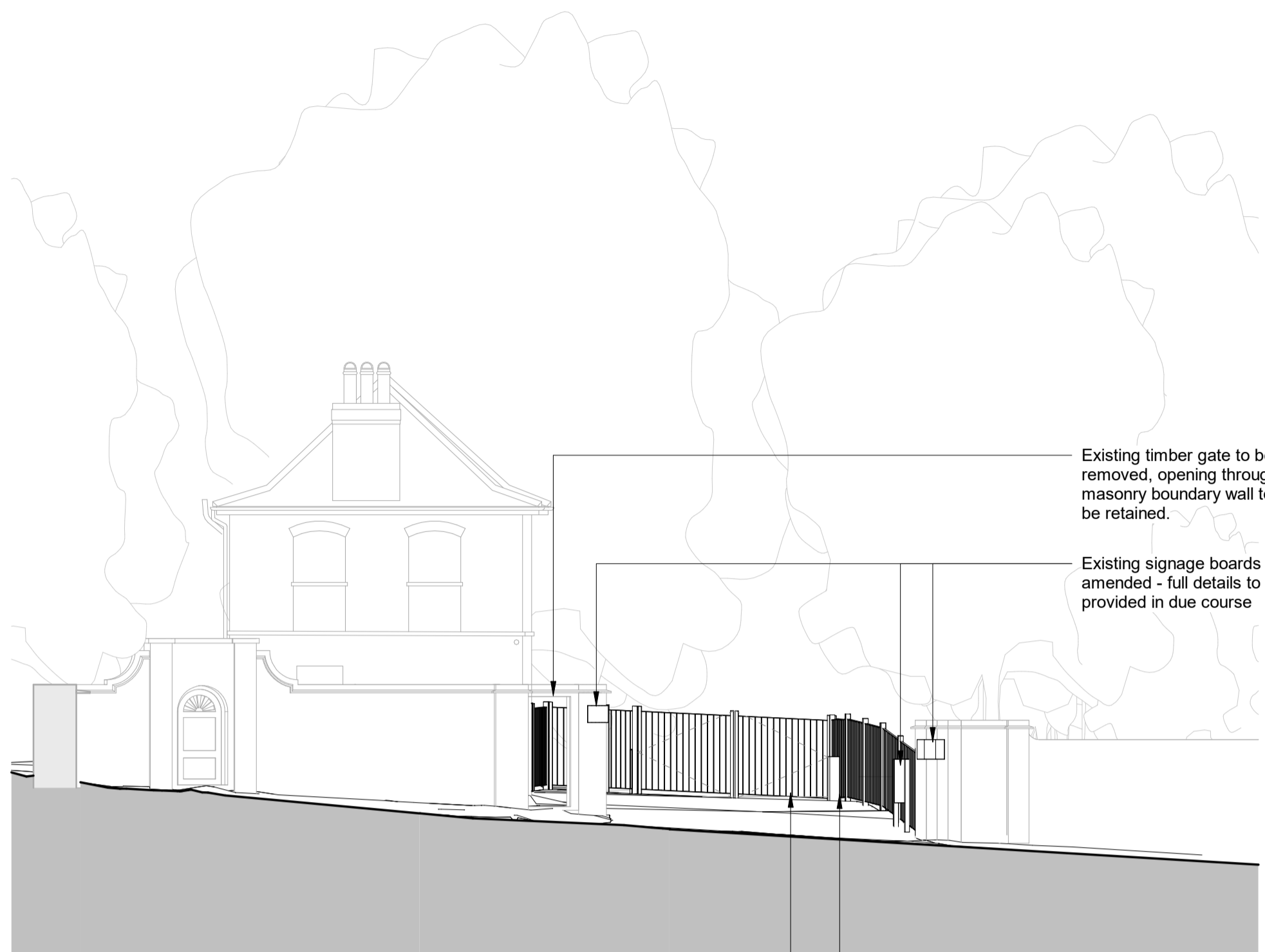
1 Site Entrance - North-West Elevation (from Queen's Road) 1:100
