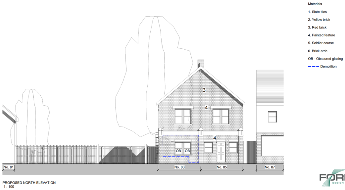
Figure 2: Proposed North Elevation of 83 Station Road.
