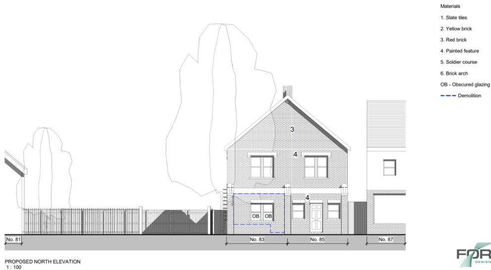
Figure 2: Proposed North Elevation of 83 Station Road.
