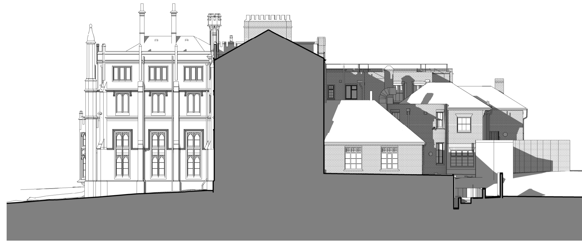
2 Main Building Section BB - Existing 1:200
