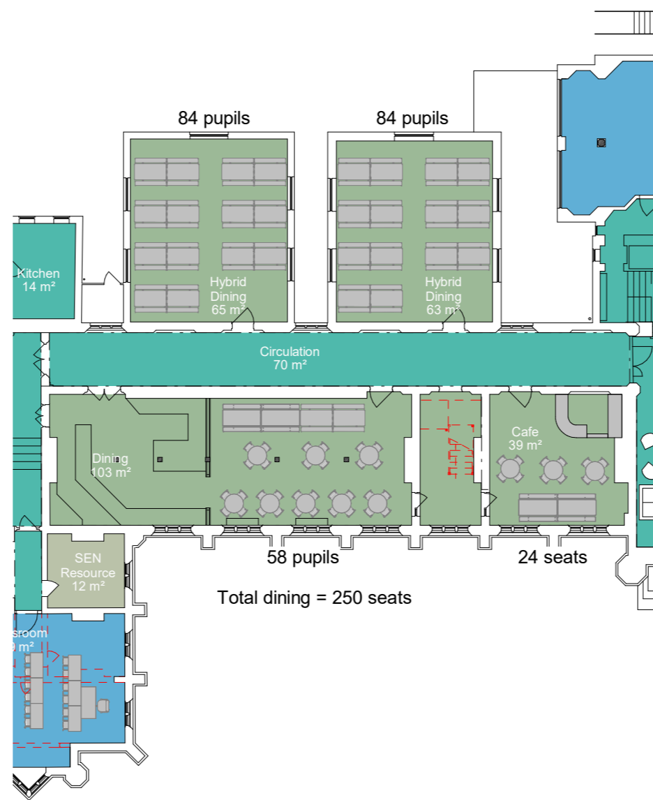
Proposed Layout - Ground floor plan extract 1:250 at A3
