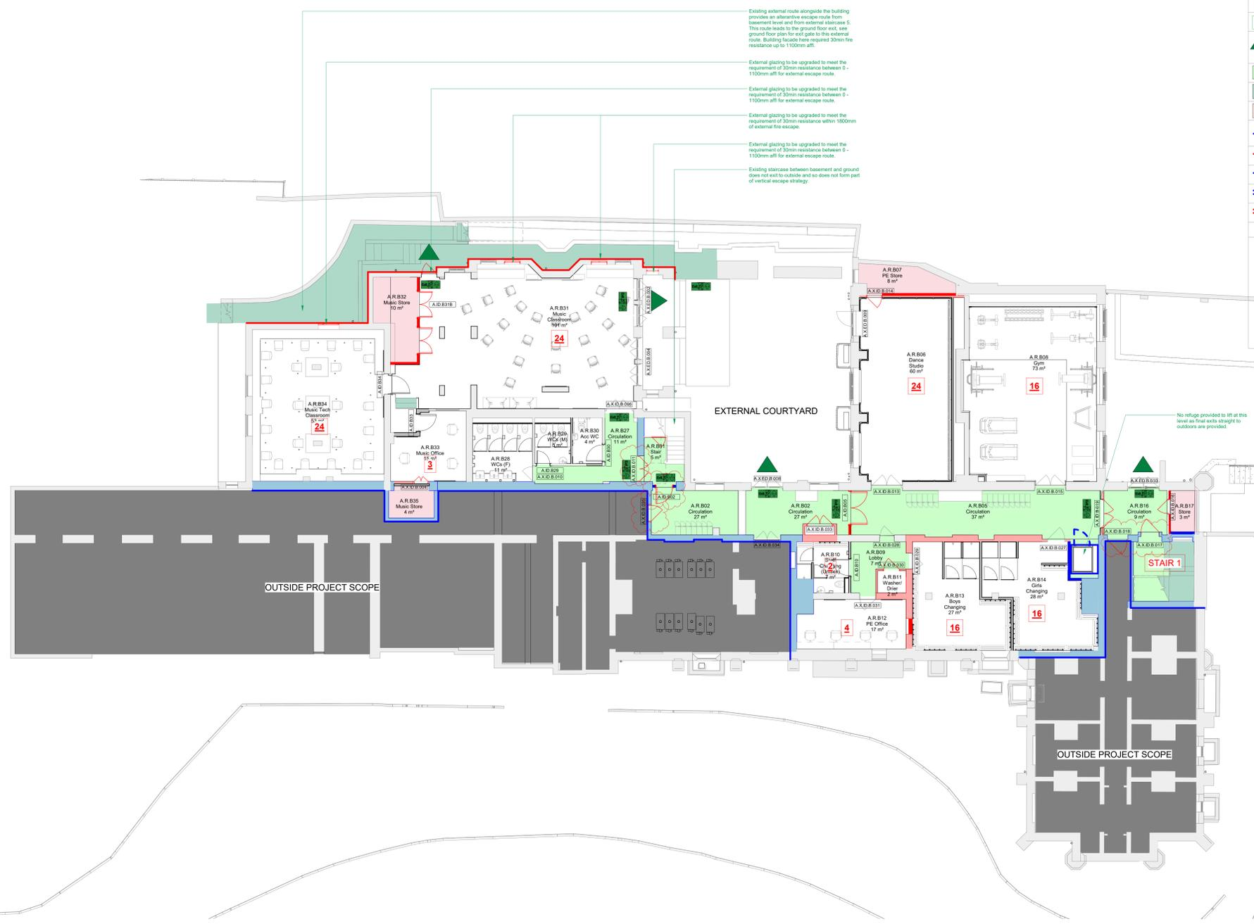
Existing external route alongside the building provides an alternative escape route from basement level and from external staircase 5. The route leads to the ground floor exit, see ground floor plan for exit gate to this external route. Building boards here required 30min fire resistance up to 1100mm a/f.
