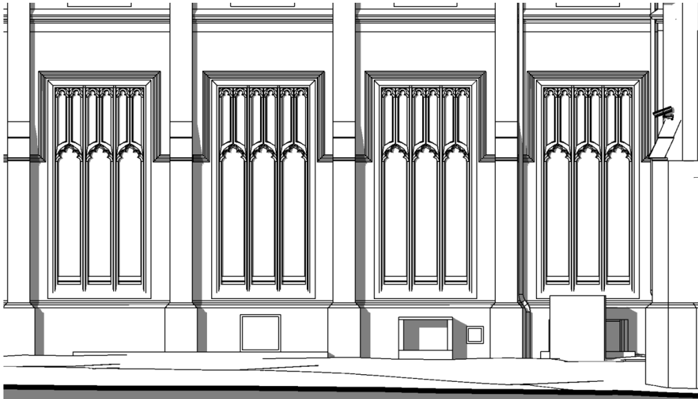
Figure 73: Detail from existing front elevation of college building – showing the part to the north of the entrance, at ground floor level. (See also Figure 75.) Note existing ventilation wall louvre, and existing external condenser plant unit and mesh framed enclosure – all at basement level.
