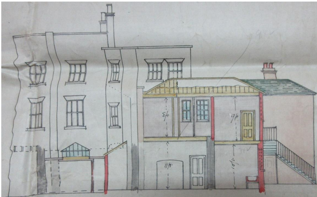
Figure 45: Section AB – proposed two-storey extension to the rear of George House, including re-modelled kitchens and new bedrooms, 1920.
