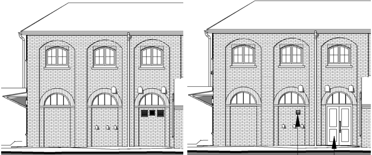
Figure 71 (left): Detail from existing Section FF – showing north-east elevation of 1920s rear extension to George House. Figure 72 (right): Detail from proposed Section FF. Note new door opening to the rear of George House (north-east elevation).
