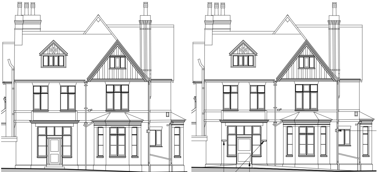
Figure 76 (left): Two-storey (plus attic storey) part of south-west elevation of The Red House – existing. Figure 77 (right): Two-storey (plus attic storey) part of south-west elevation of The Red House – proposed.
