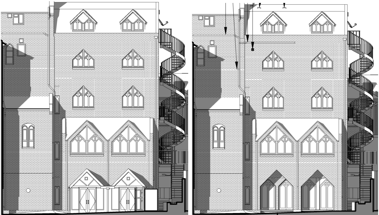
Figure 69 (left): Detail from existing Section DD – showing north-west elevation of rear extension B. (See also Figure 68.) Figure 70 (right): Detail from proposed Section DD. Note removal of modern “conservatory” to 1980s extension (labelled B in Figure 56).
