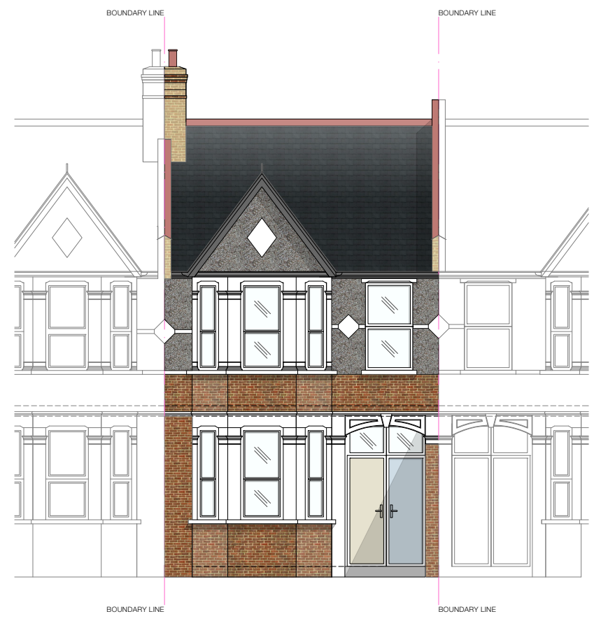
4 Existing Front Elevation 1:100 @ A3
