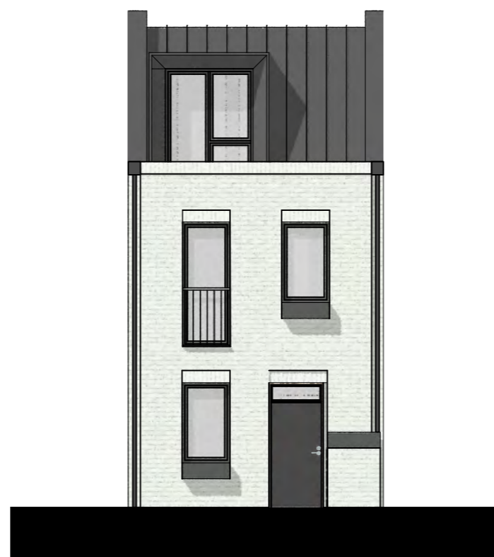
A2 Front Elevation White Painted Brickwork Scale: 1:100
