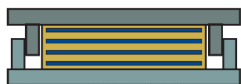
Figure 5. Concept of restraint plates either side of elastomeric bearing to provide transverse fixity
