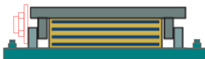
Figure 6. False roller end plate with protruding threaded stud and nut attached to restraint plate (shown in red)
