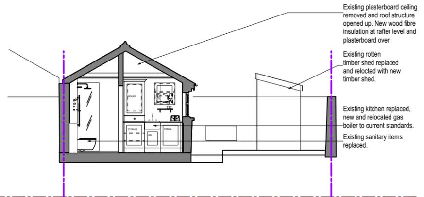
**1 SECTION / ELEVATION E-E AS PROPOSED**
