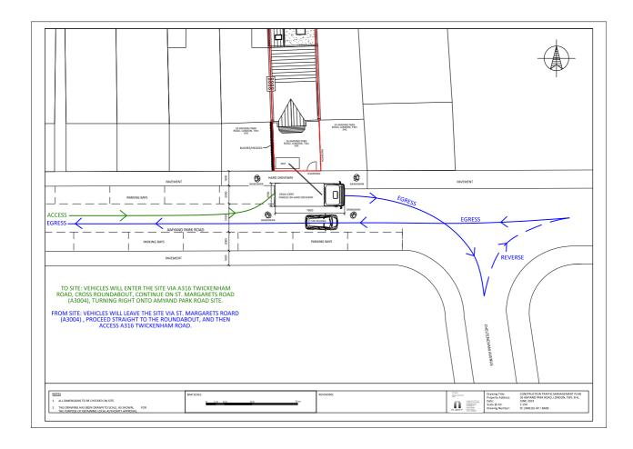
All delivered materials will be stored within the curtilage of 26 Amyand Park Road. It is proposed that general site waste will be disposed within the secured, hoarding (2.4m heigh). No plant will be stored on the public highway. It is proposed that excavation spoils will be deposited into a skip placed within the curtilage and a wait and load method of spoils removal be used.
