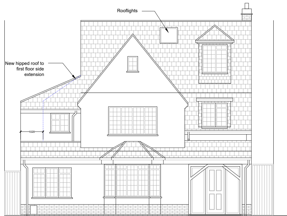
01 Proposed Front Elevation 1:100 @ A3
