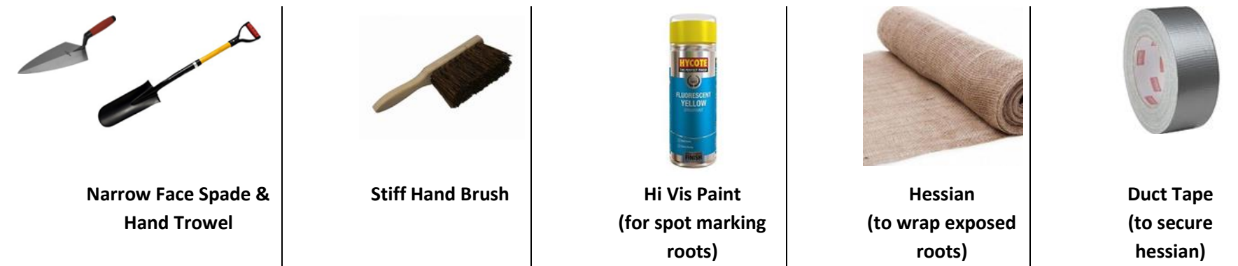
Fig 14 – Advised tools/ materials which should be available for all excavation works within RPA
