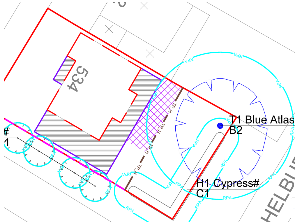
Fig 8 – Temporary ground protection will be used to be realistic to construction movements on site (hatch).
